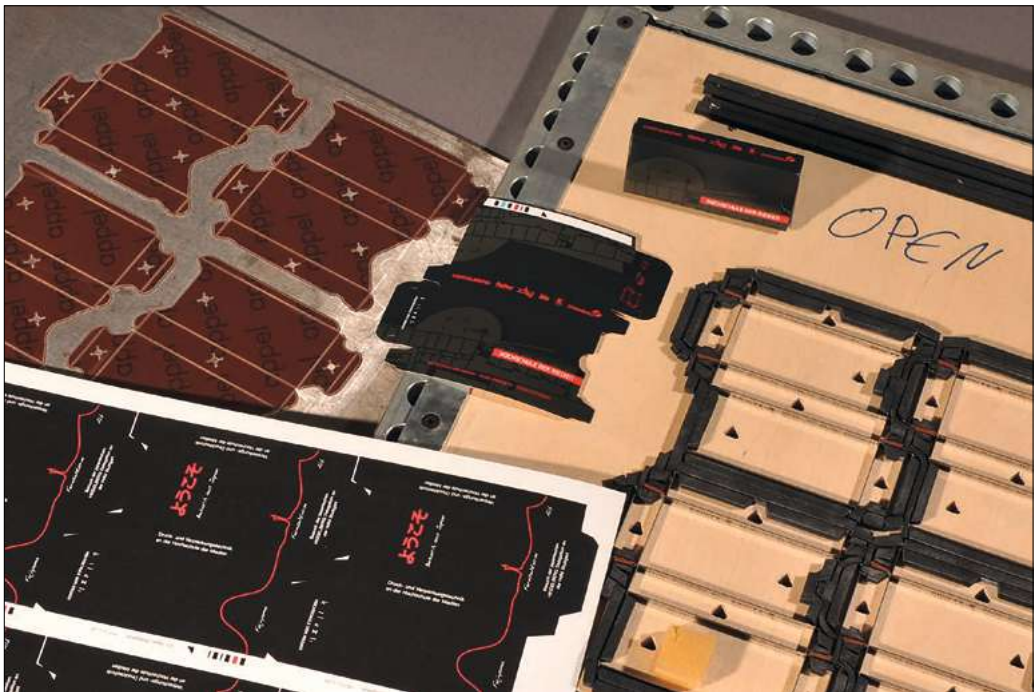
Figure 12.3 Elements of a die: rubberized die in closed frame (right), die plate with counter punch (top left), press sheet (bottom left), punched and broken- out single unit (center), and finished carton
